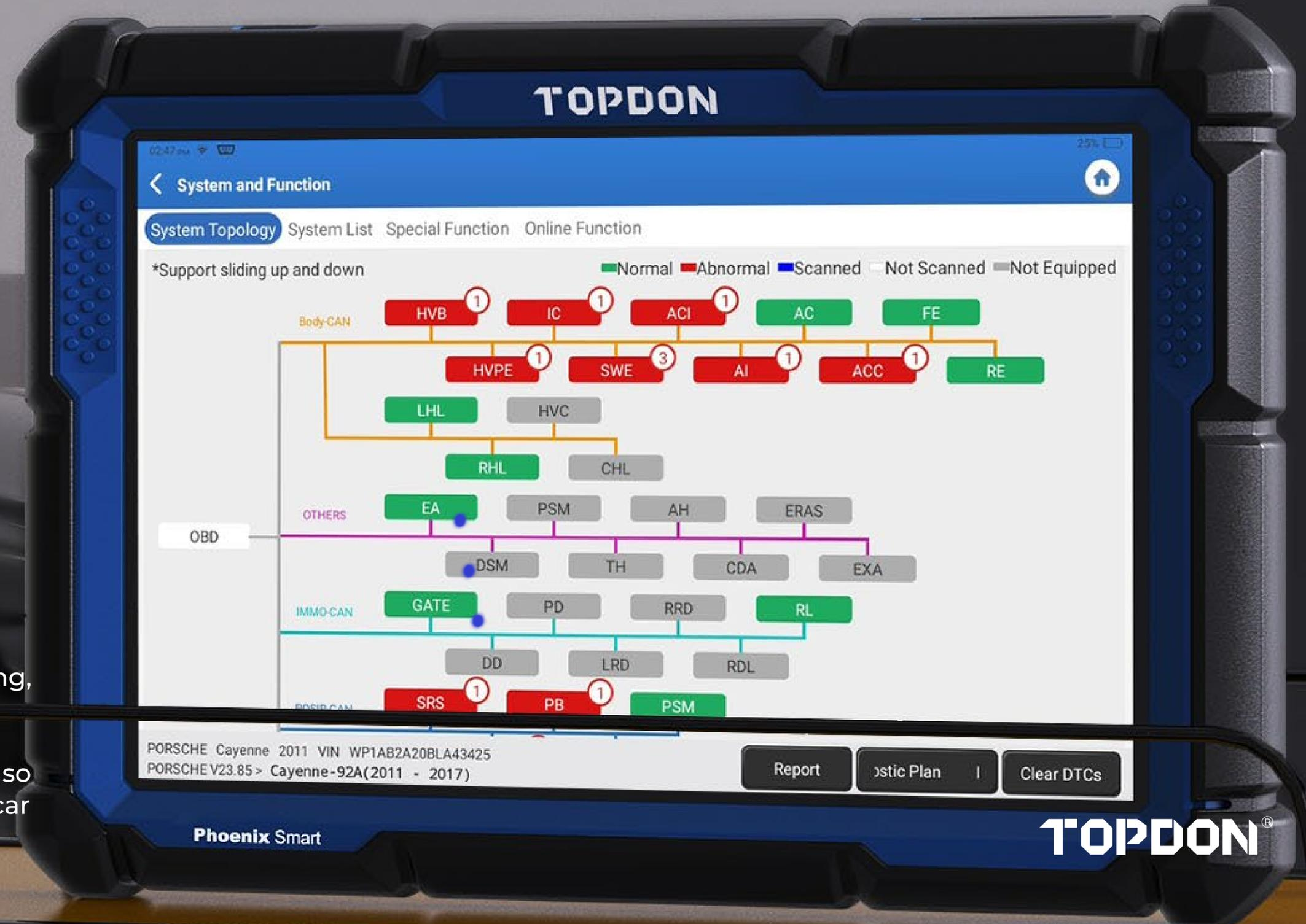
The Phoenix Smart Utilizes Topology mapping, displaying the entire vehicle system.
